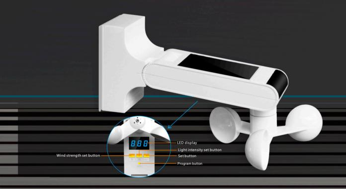
Power supply Solar panel +DC 3.7V lithium battery Working temp -40°C ~ +85°C Frequency 433.92MHz
